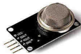
Fig.5 Air checking purity sensor (MQ135)
